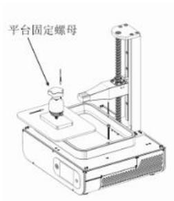
a) insert platform and fix it tightly , Rock the platform with your hand and make sure it has been loosened
